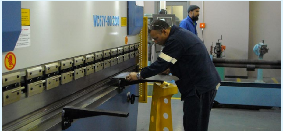
Fadiel Rycliff, an ARPL candidate and employee of the company 3C Metal, operates a press brake machine. A press brake is a machine pressing tool. It is used for bending sheet and plate material, but usually sheet metal. It is utilised for forming pre-determined bends by placing the workpiece between a matching punch and die or a V Block and Bending Blade. The high-tonnage hydraulic press brake featured here, forms part of the top-end training equipment used by the college. Candidate artisans practice their practical tasks using this, and related, specialised equipment
