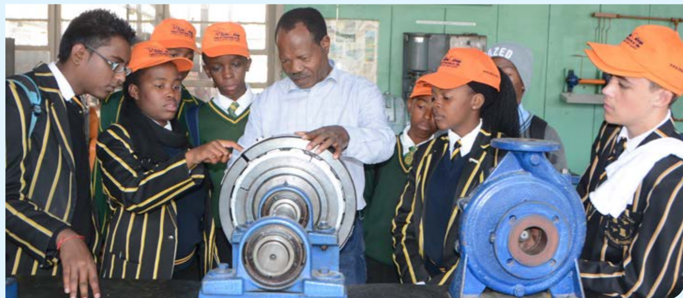
Training Officer at Newcastle Training Centre, Mr Joe Mfaba, provides a detailed explanation in the Mechanical Workshop, to Newcastle High School learners, on how the Cooper Split Bearing works
